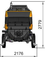
Note: Standard version BSA 2110 HP D5. Dimensions and weights depend on equipment. Subject to technical modifications and errors.
