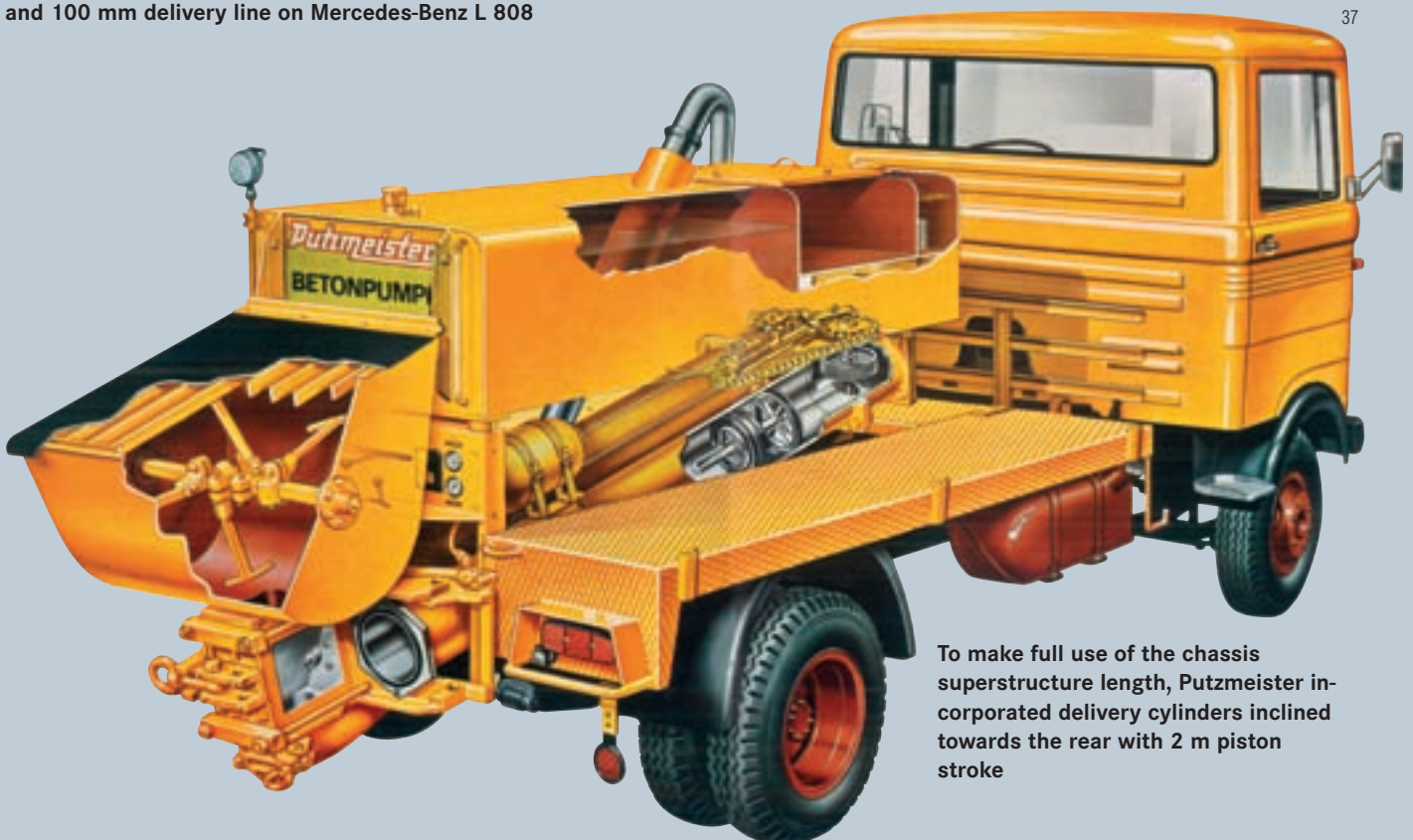
First Putzmeister truck-mounted concrete pump with M 16 boom and 100 mm delivery line on Mercedes-Benz L 808
