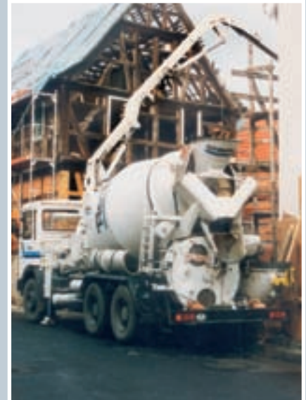
The Wibau truck mixer concrete pumps with rotor were in competition with the Putzmeister PUMI® with piston pump in the second half of the 1980s
