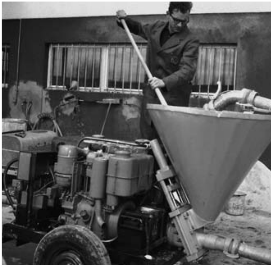
Trials are performed by the boss himself: in 1966, KS tests his first oil-hydraulically driven concrete pump HB 1 with flat gate valve, for pumping fine concrete and screed
