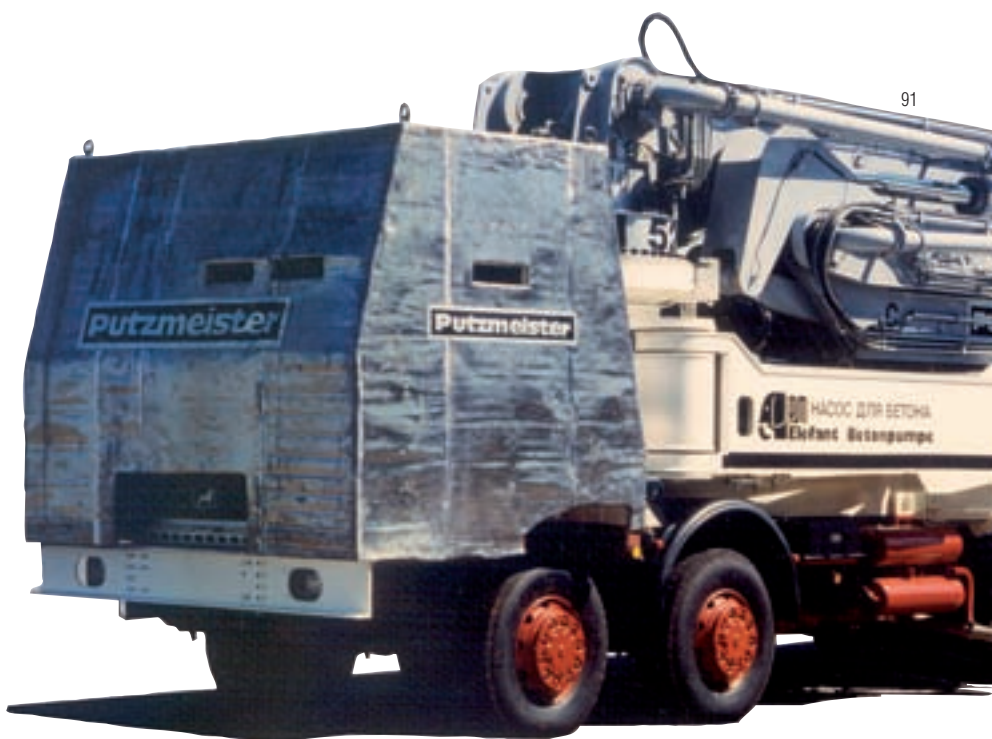
For their work in Chernobyl, truck-mounted concrete pumps were equipped with protective lead covers and remote-controlled video cameras for the first time
