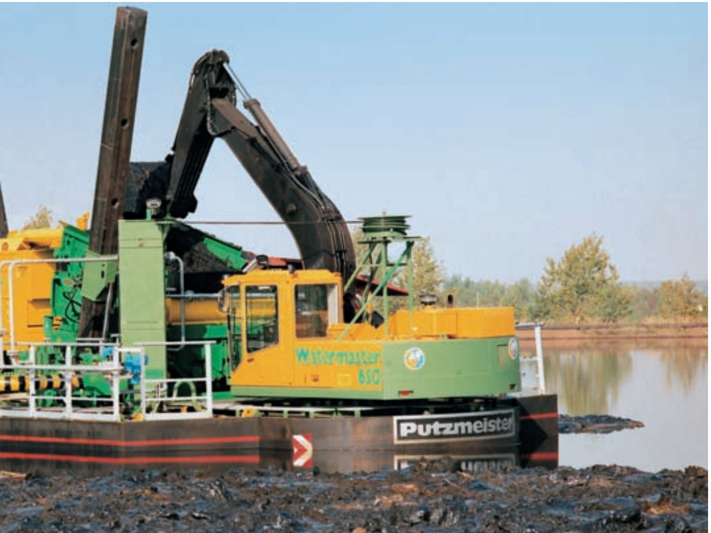
For land reclamation – as here off the Japanese coast – particularly high-capacity Putzmeister high density solids pumps with an hourly output of 500 m 3 are used
