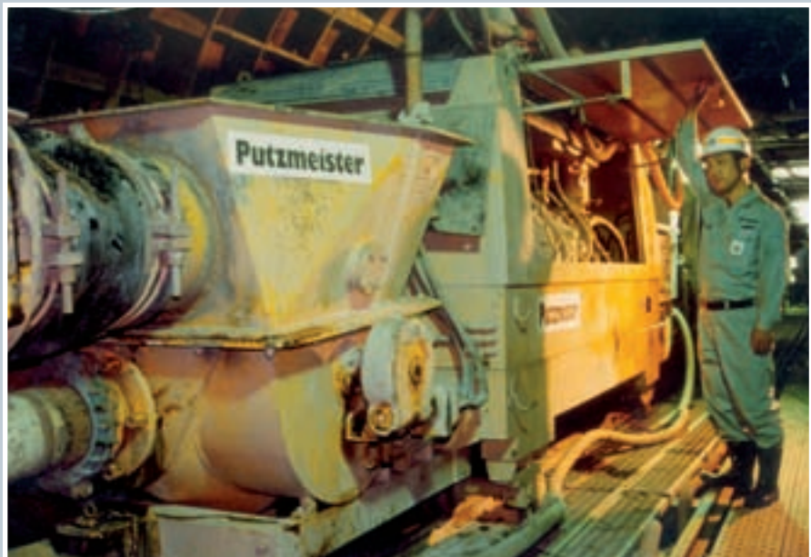
This Putzmeister concrete pump pumped waste excavated from the tunnel during the construction of the Tokyo underground
