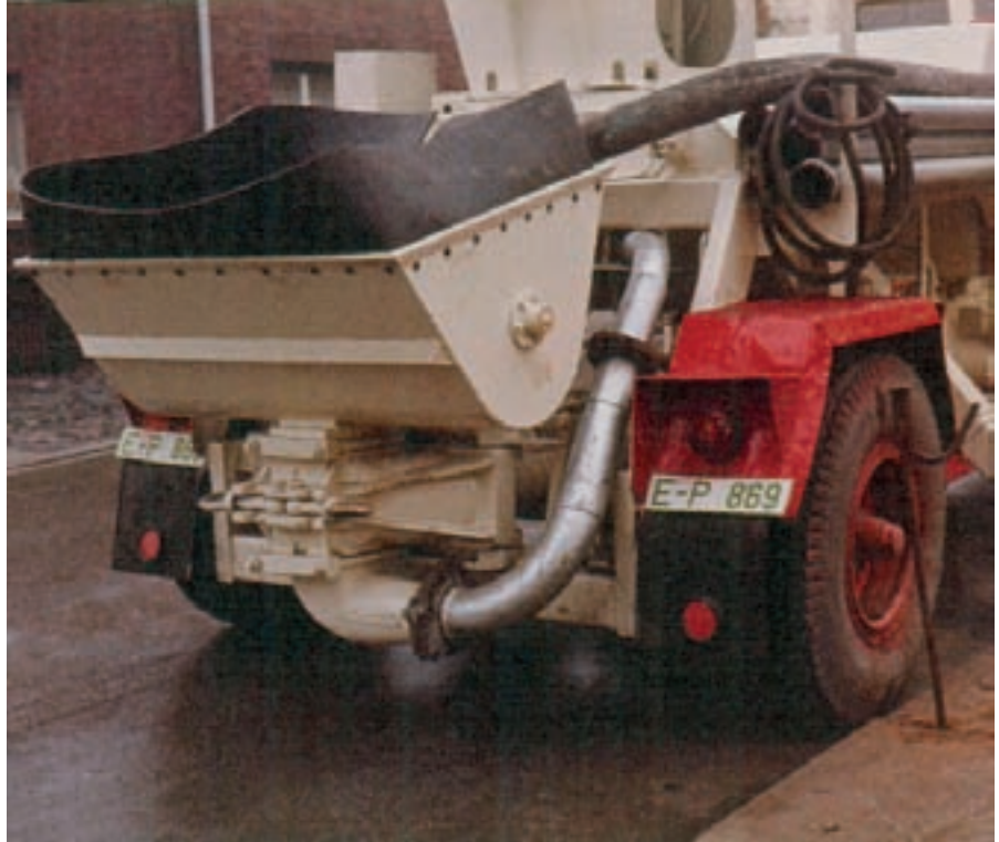
Hostadt conversion: Take a Torkret truck-mounted concrete pump with gate valve and replace the power unit with a water hydraulic Putzmeister pump with flapper system... (Ill. Hostadt)
