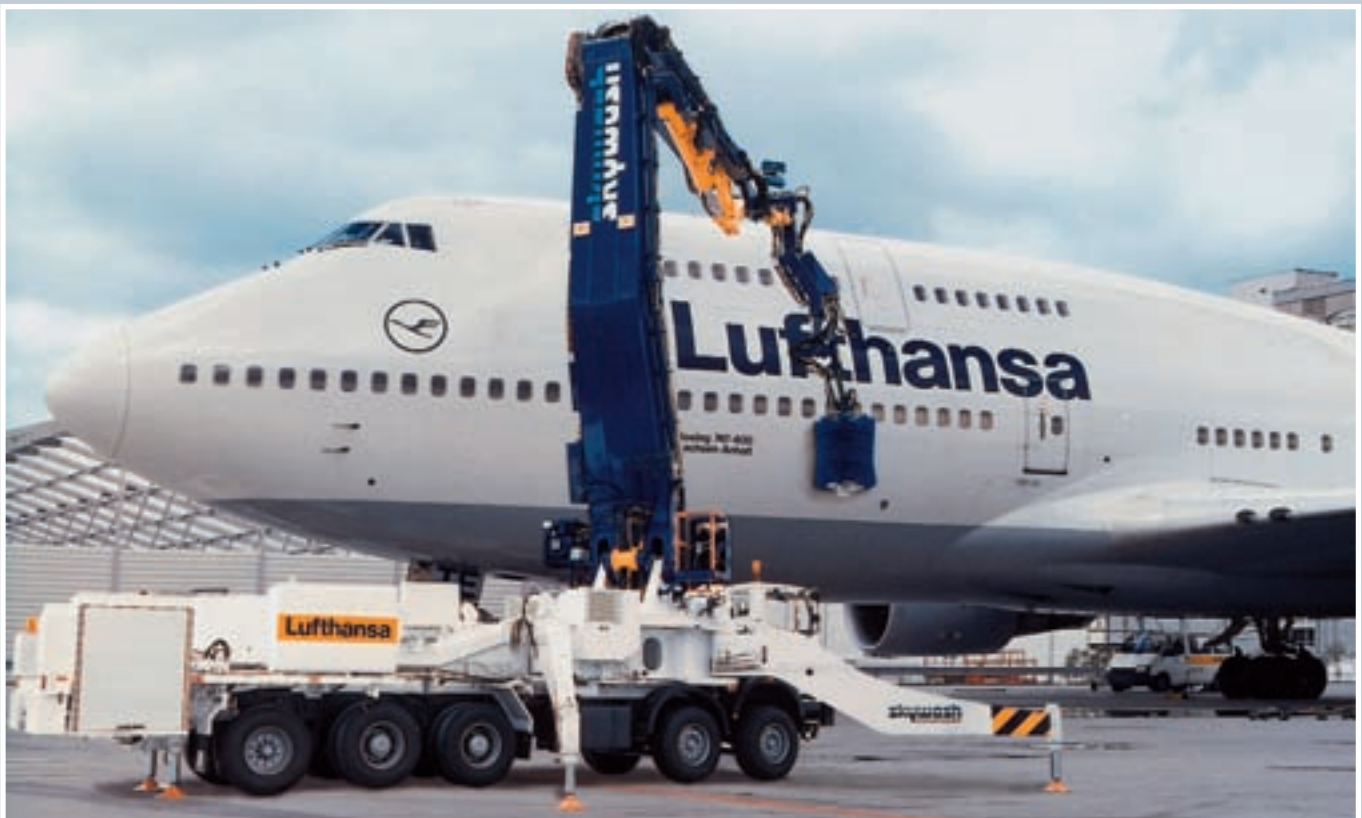
Two of these large mobile robots clean a Jumbo in two hours
