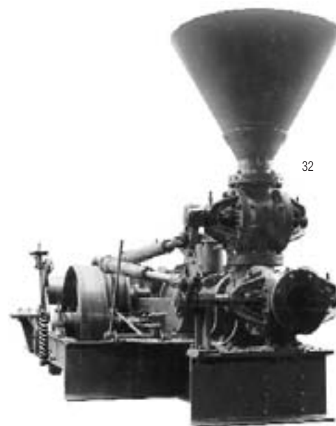
Torkret concrete pump with horizontal cylinder and spring telescoping slide rod, below in a systematic diagram, Kooymann System (Ill. Torkret)
