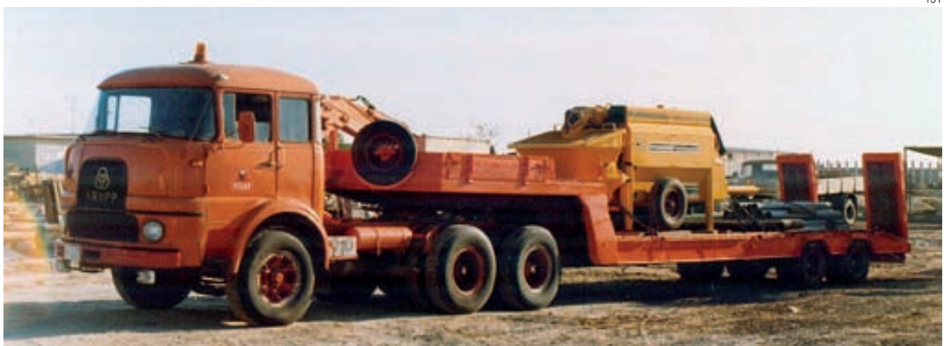
A Krupp semi-trailer vehicle brings the new stationary Putzmeister concrete pump to the construction site. The photo is from circa 1980. (Ill. Eller)
