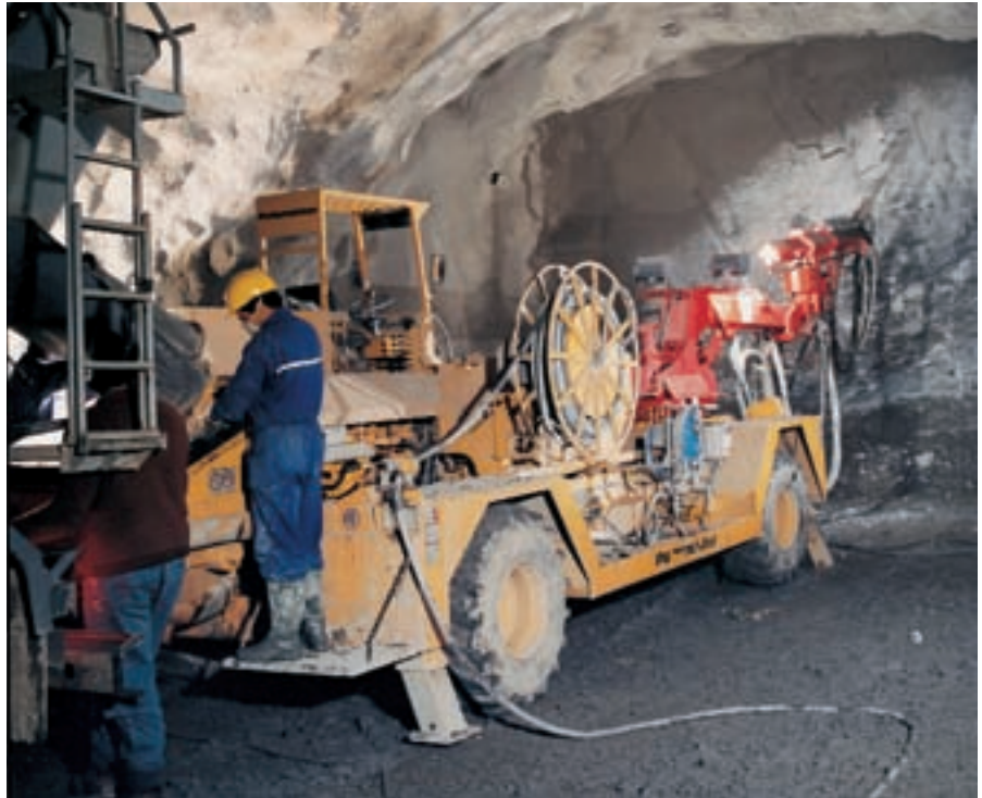
In the 90s, PMIB had specialised in wetcrete spray concrete machines. They were seen as successors to the large German-produced Putzmeister spray buffalos.
