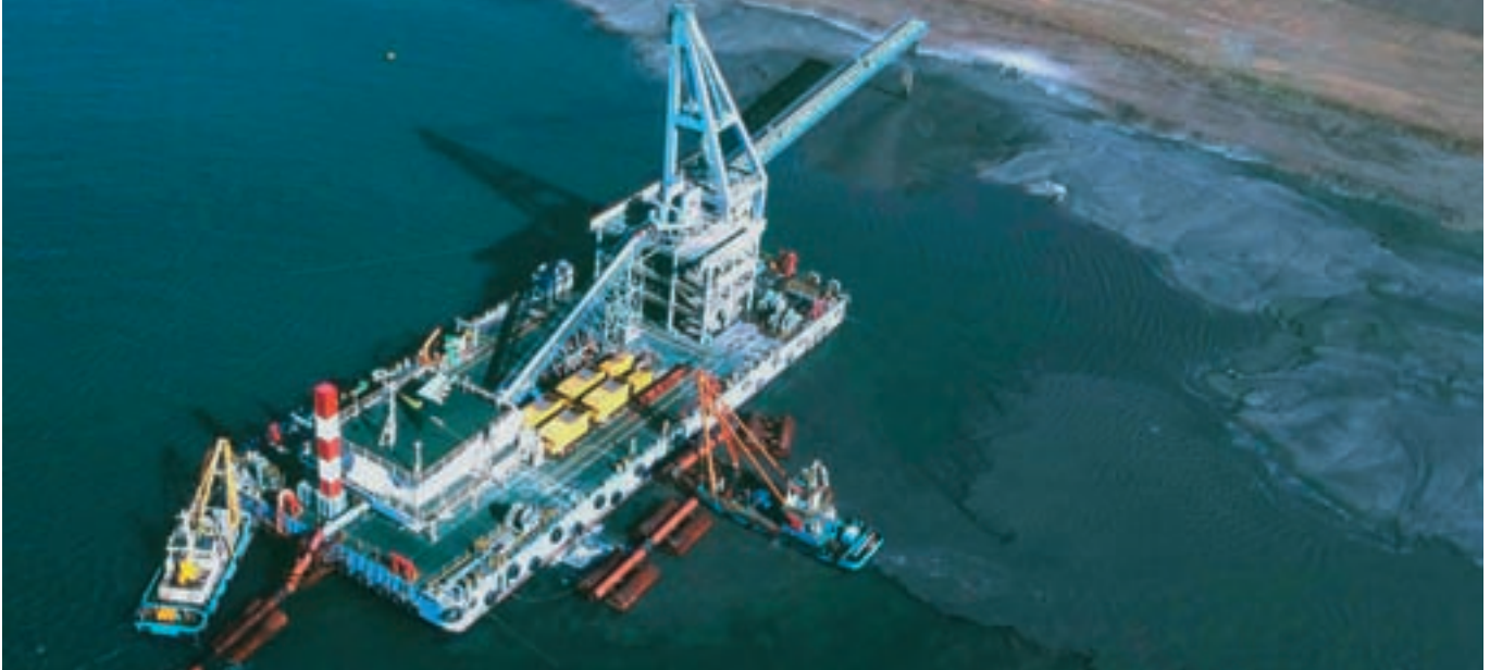
For land reclamation – as here off the Japanese coast – particularly high-capacity Putzmeister high density solids pumps with an hourly output of 500 m 3 are used
