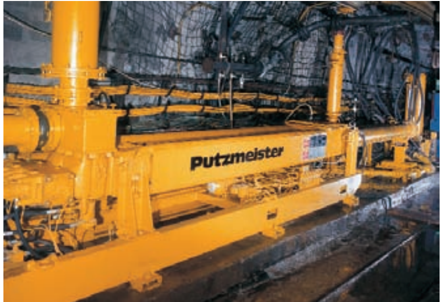
This large high density solids pump is controlled via seat valve and pumps gritty mine water out of a mine in Lorraine
