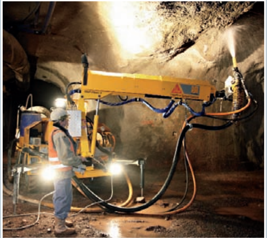
Compact concrete wet spraying machine from the Sika-Putzmeister alliance for tunnels and galleries with a small cross section
