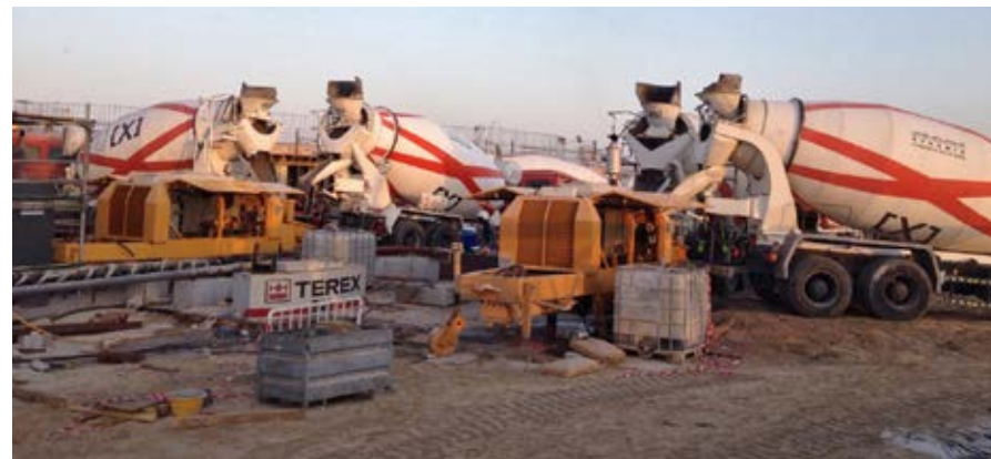
► The two BSA 2110 HP D pump a total of 65,000 m 3 of concrete for this project
