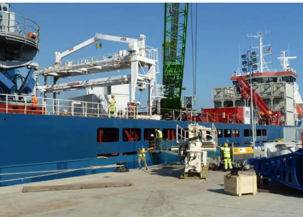
▼ The arm assemblies for the stationary booms were hoisted onto the ship in the Port of Rostock...
