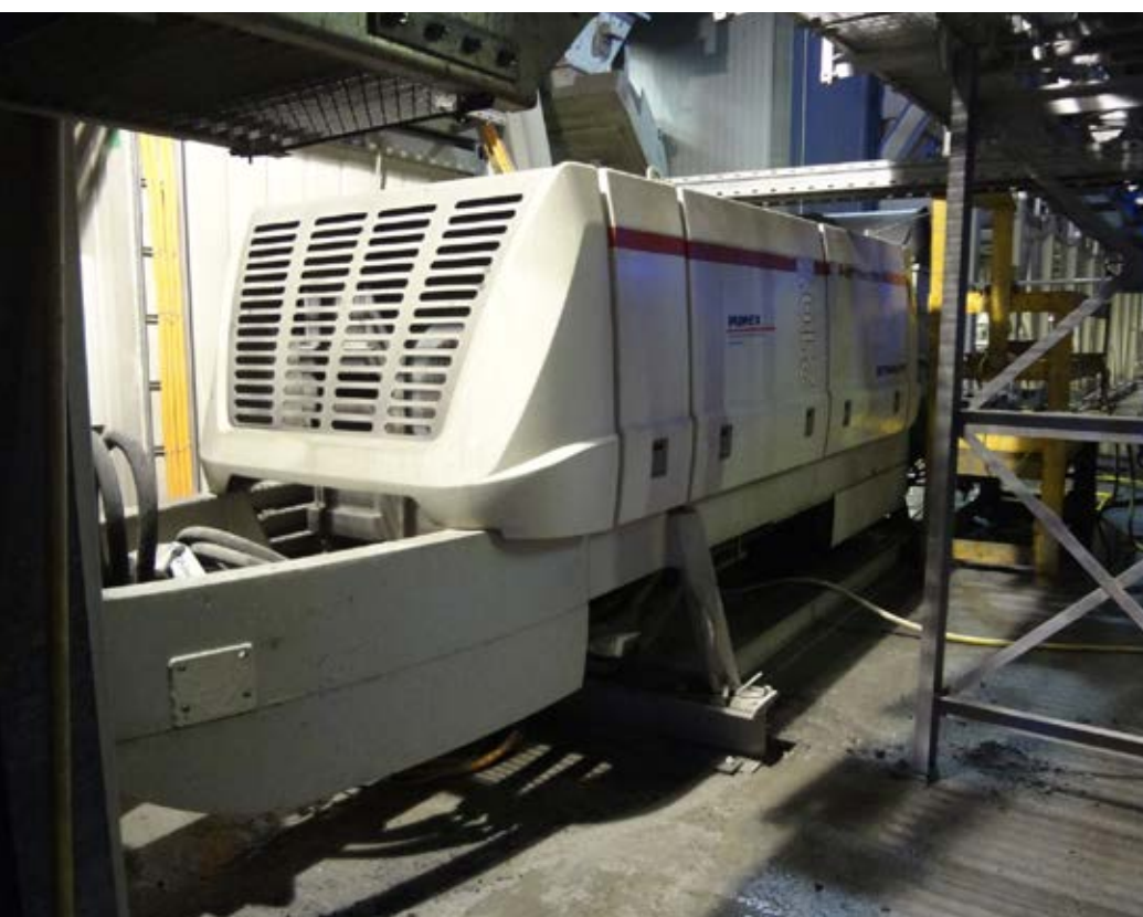
▼ The BSA 2107 HPE stationary high-pressure concrete pump under the mixer
