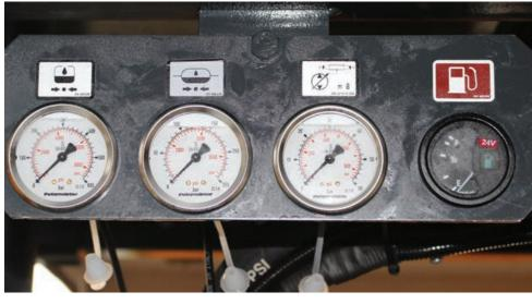
Mini-measuring strip: All hydraulic measuring points at a central location (BSA latest generation)
