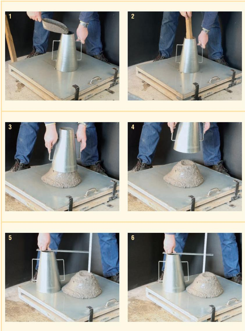
Fig. 11: Measuring slump in accordance with DIN EN 12350-2
