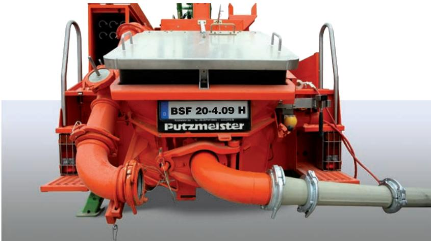
Fig. 30: Reduction from DN 150 to DN 65
