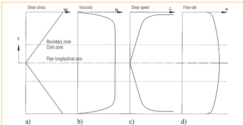
Fig. 26: Flow influences on the pipe conveying of fresh concrete
