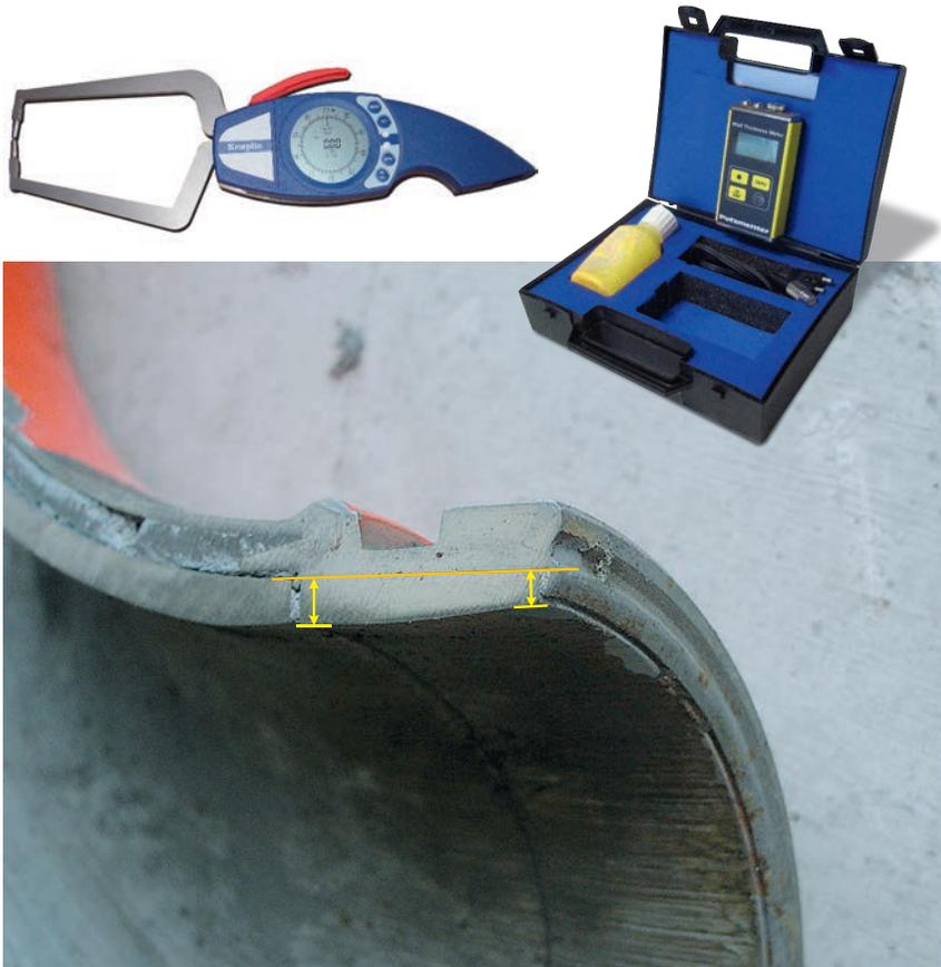
Fig. 32: Measuring pipe wear: wall thickness measuring units for two-layer lines (le.) and single-layer lines (ri.)
