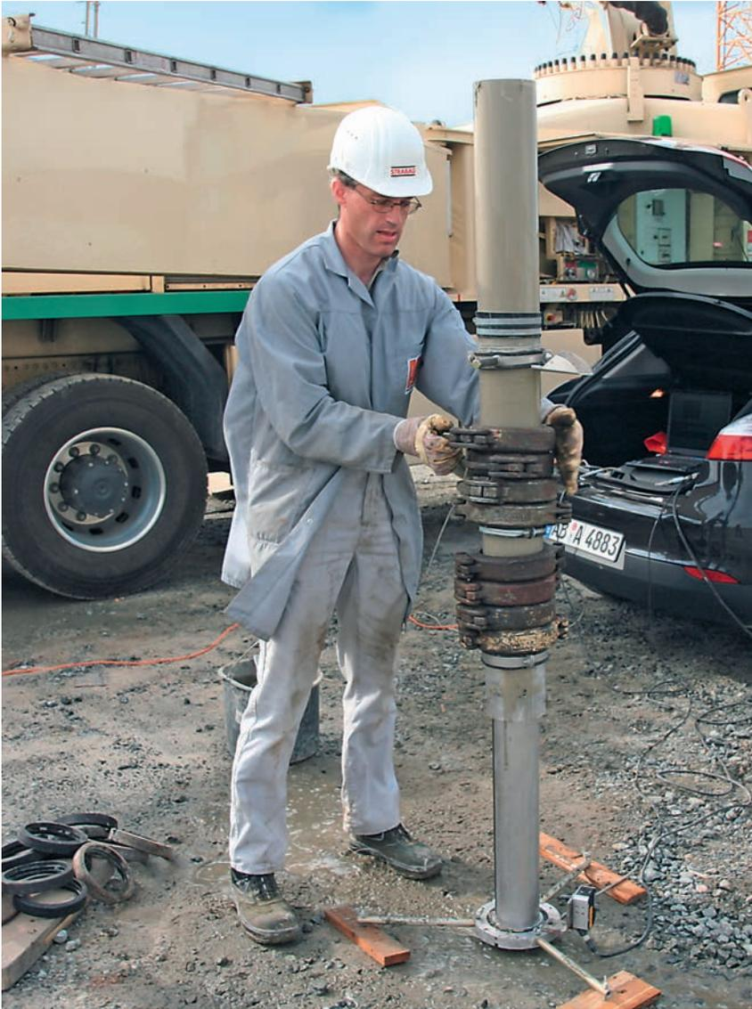
Fig. 34: Measuring the consistency coefficient of freshly-mixed concrete using the Sliding Pipe Rheometer
