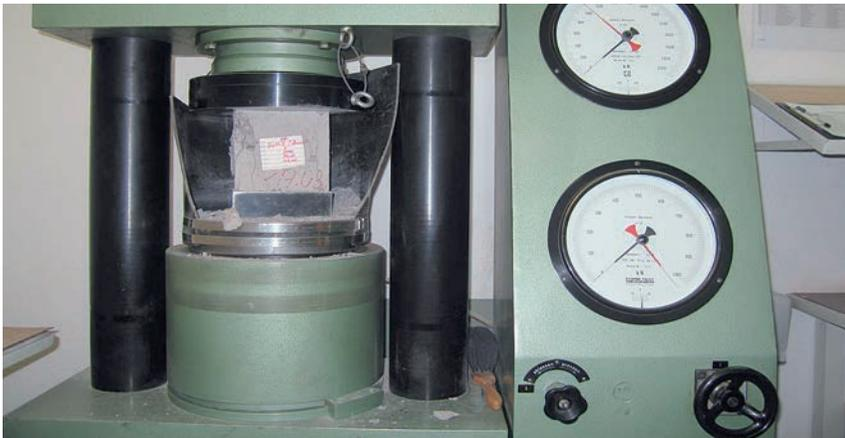
Fig. 16: Compressive strength test
