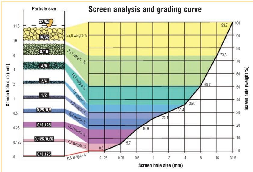
Fig. 3: Sieve analysis and grading curve
