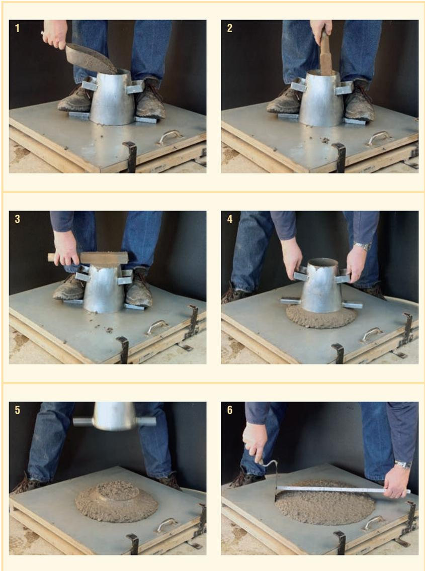
Fig. 10: Measuring spread in accordance with DIN EN 12350-5
