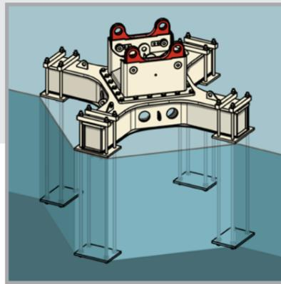
Attached on a base plate with anchors embedded in the foundation <sup>(2)</sup>
