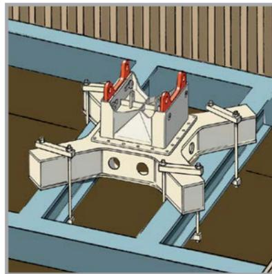
Cruciform base mounted on a shaft frame with tie-rods <sup>(6)</sup>
