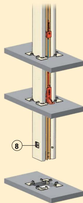
When climbing starts, the swing claw holds the placing boom up, while the lifting cylinder retracts for the next lift.
