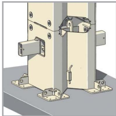
RS-850 with existing base plate and slab fixed with four base plates <sup>(4)</sup>
