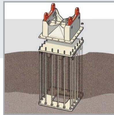
Compact cruciform base anchored in the foundation with a tie-rod cage (when space is restricted) <sup>(3)</sup>
