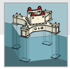
Attached on a base plate with anchors embedded in the foundation (2)
