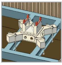
Cruciform base mounted on a shaft frame with tie-rods <sup>(6)</sup>
