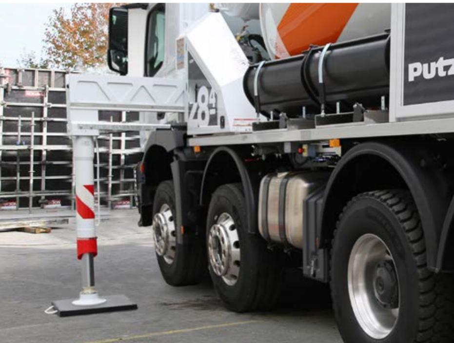
The unique variable support offers a long reach and a high level of safety even in confined setup conditions
