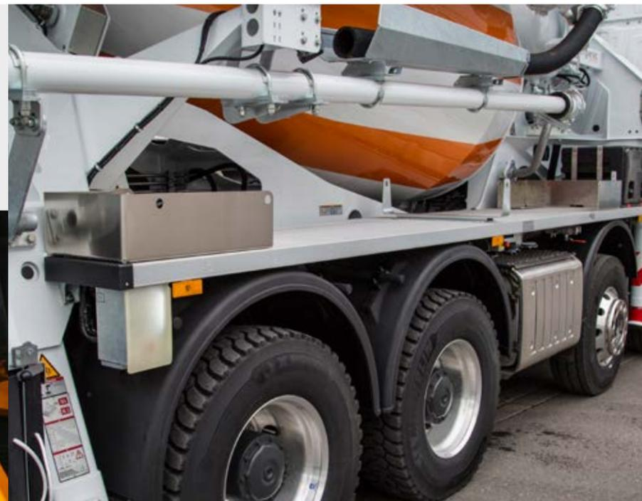
Continuous and flat user-friendly platform with plenty of space for hoses, base plates, chutes etc.
