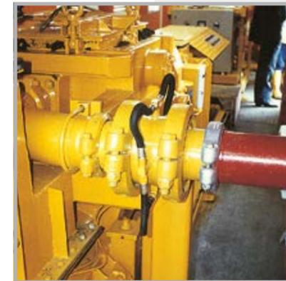
The injection of water or lubricants significantly reduces the pressure loss in the delivery line Example: Sewage sludge with 37% and up to 47% dry solids content
