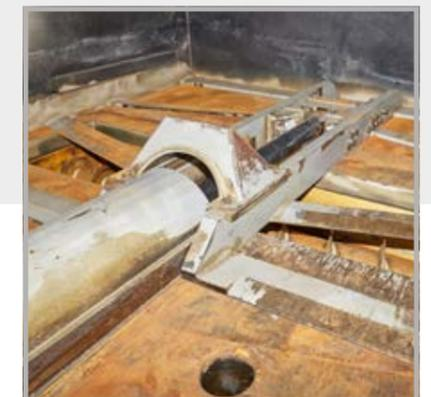
PDL rectangular discharge sliding frame
