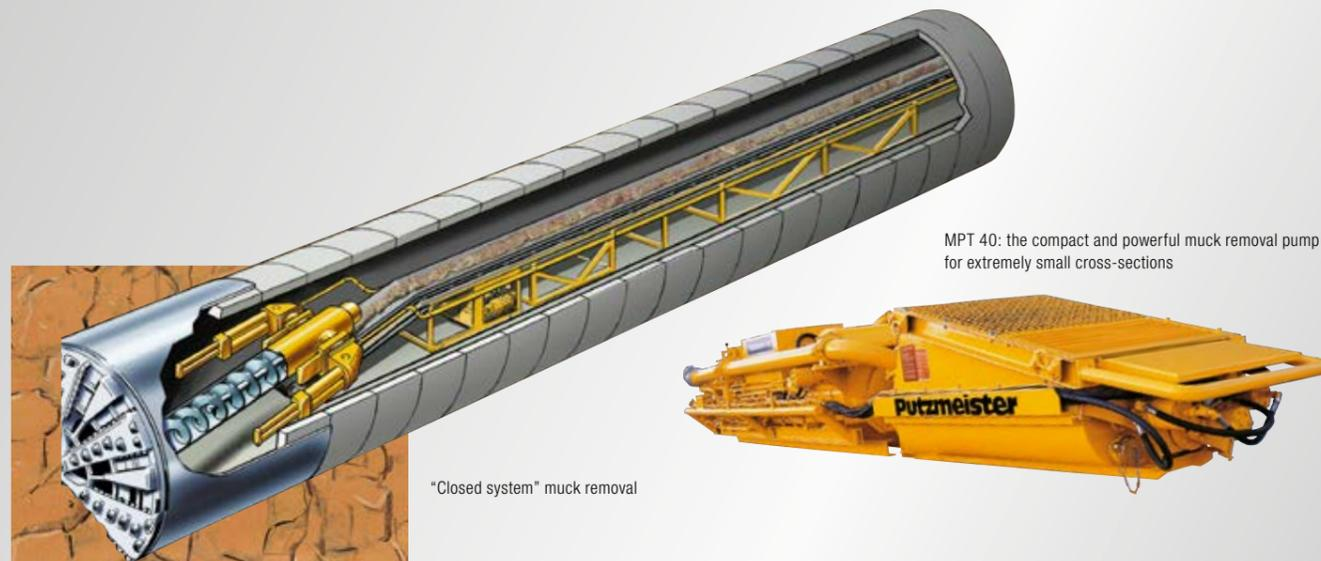
MPT 40: the compact and powerful muck removal pump for extremely small cross-sections
