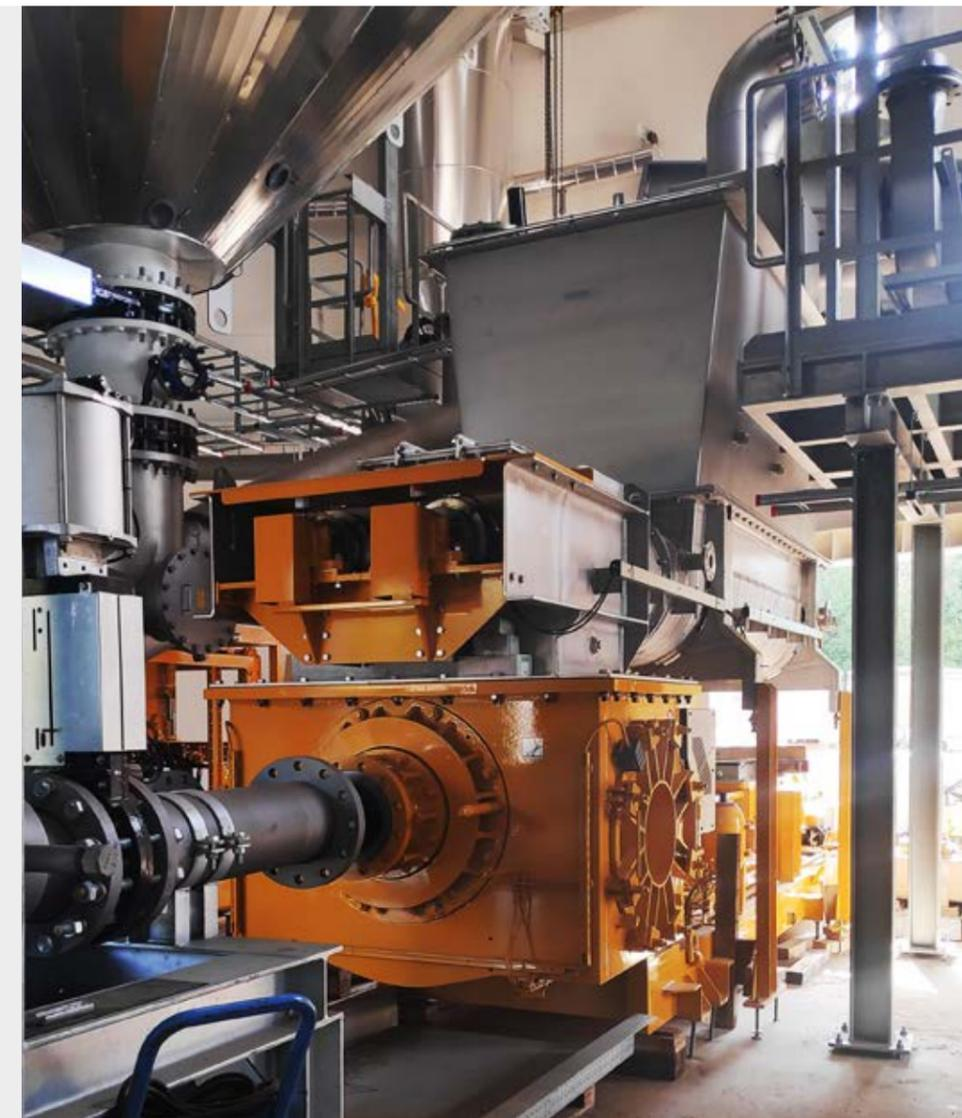
KOS 25100 with hydraulic power pack and twin-screw feeding device, transporting biomass to the fermentation tank
