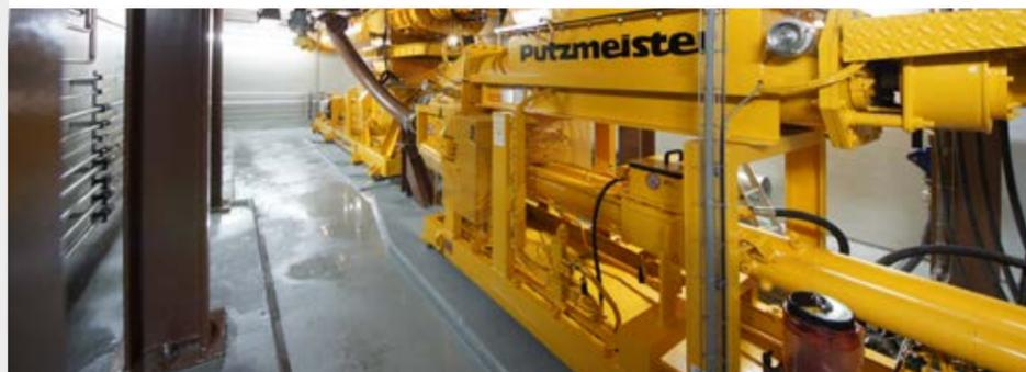
Background: KOS 1080 piston pump under a 30 m<sup>3</sup> receiving bunker. Foreground: KOS 1030 piston pump to feed the kiln lines under a 230 m<sup>3</sup> storage silo. Installed in a very narrow former waste bunker.
