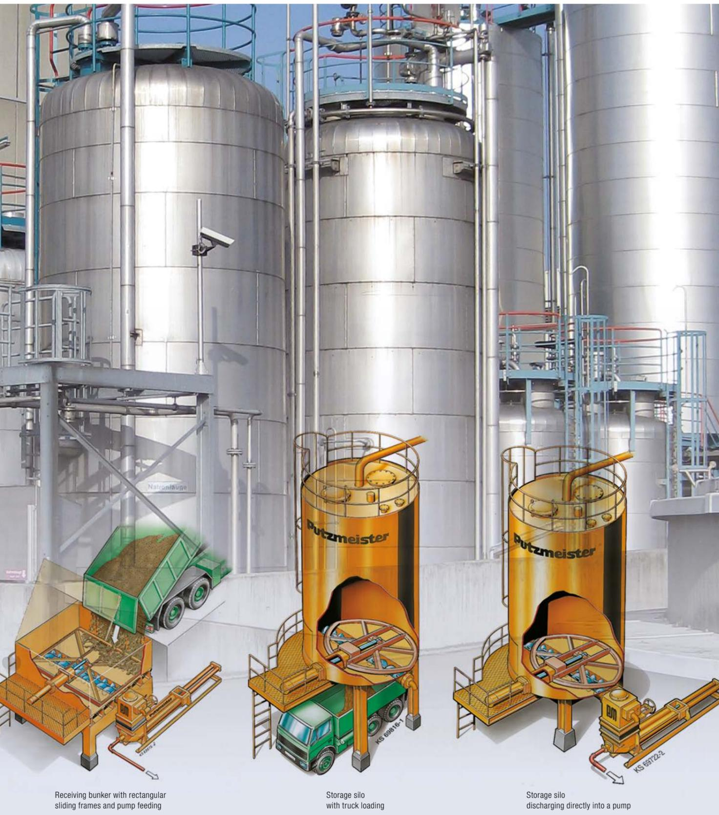
Receiving bunker with rectangular sliding frames and pump feeding
