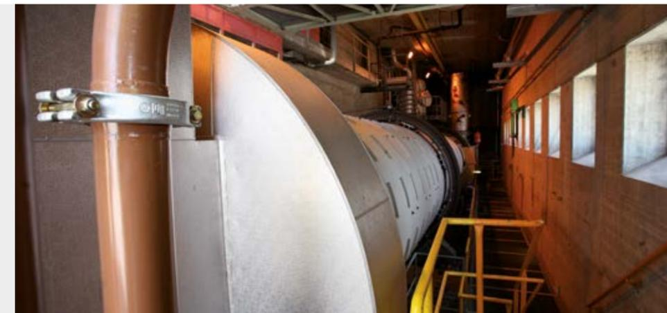
Erzo Oftringen sewage treatment plant (Switzerland): rotary kiln for the incineration of sewage sludge
