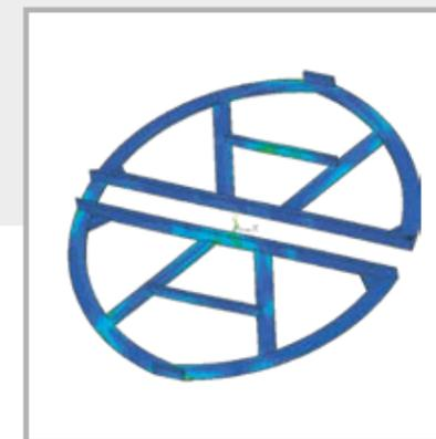
Finite element analysis for the sliding frame
