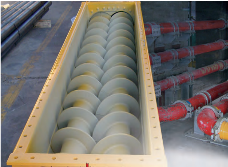
Fig. 119: Double feeding screw
