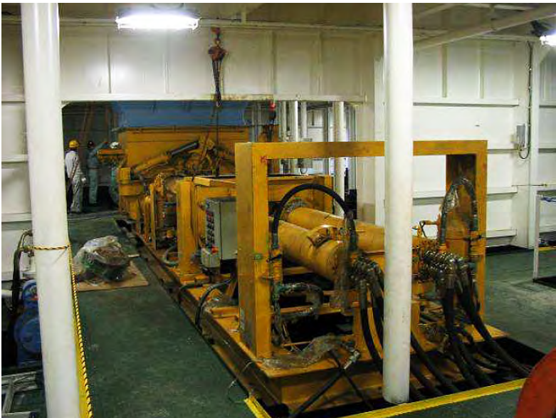
Fig.72: Piston pump- installed below deck
