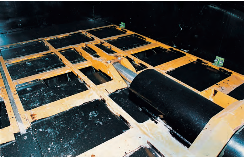
Fig. 100: Sliding frame for rectangle bin
