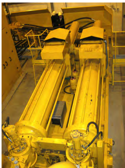
Fig. 47: Large volume piston pump HSP 25150 HP
