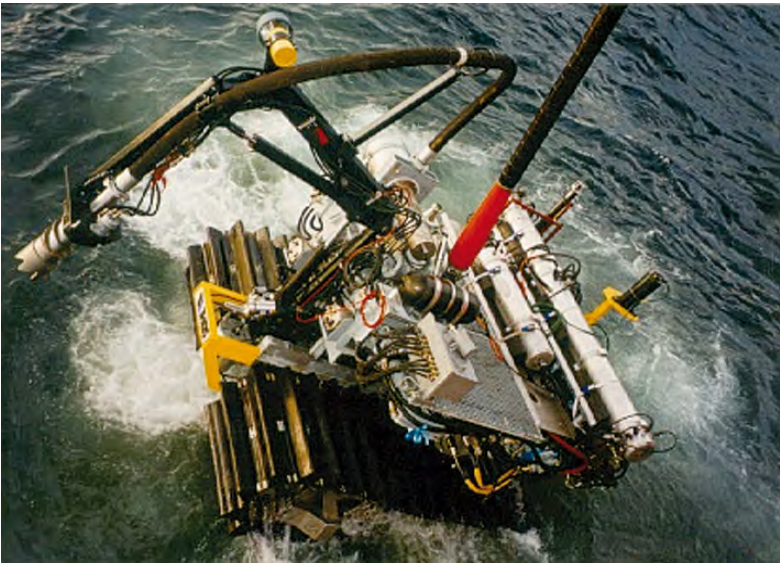
Fig. 69: Subsea pump is left to water
