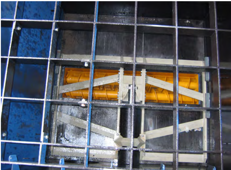
Fig. 112: Look in the bunker with rectangle sliding frame 3.5 x 3.5 m (LxW) and auger feeder (yellow) 2 x 400 mm diameter with 3.5 m length
