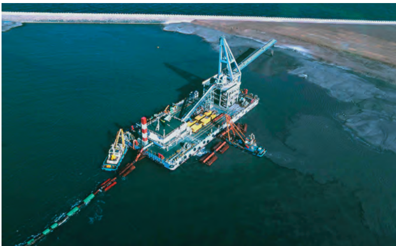
Fig. 147: Sludge supply with barge preparation plant on the vessel stacker conveyor for the prepared medium
