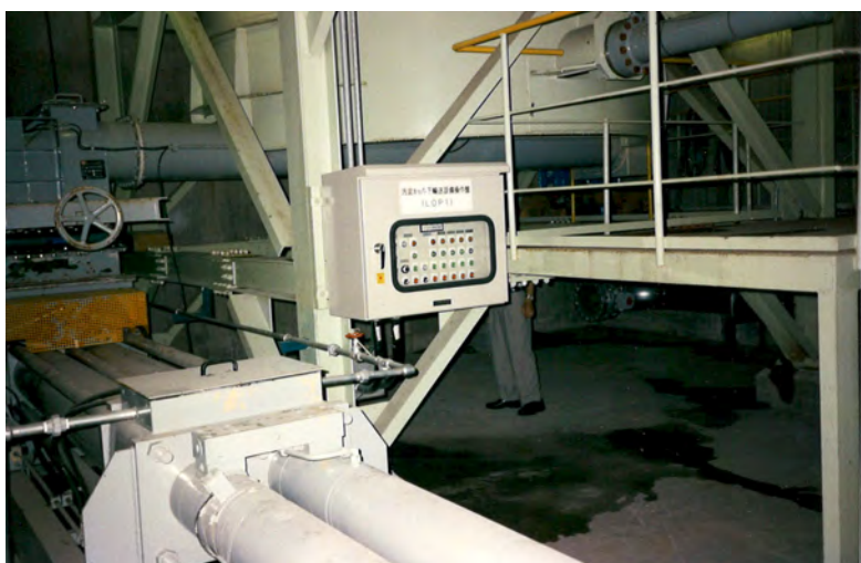
Fig. 102: The construction height can be minimized with the double combing pre-pressing screw
