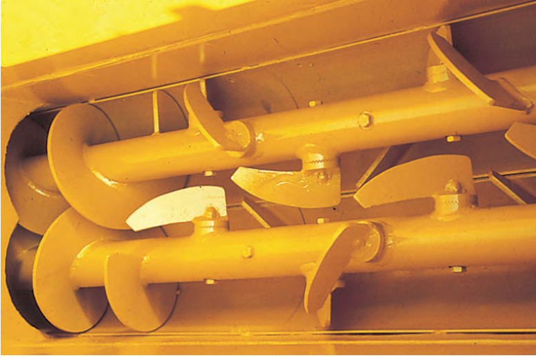
Fig. 115: Double pre- compression screw with mix blades
