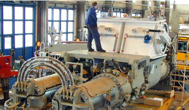
Fig. 66: High-density solids pump in twin version with pressure resistant hopper
