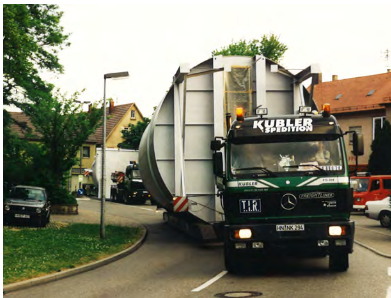
Fig. 106: Transport of the complete manu- factured silo with 5.5 m diameter and 13 m total length to the installation side
