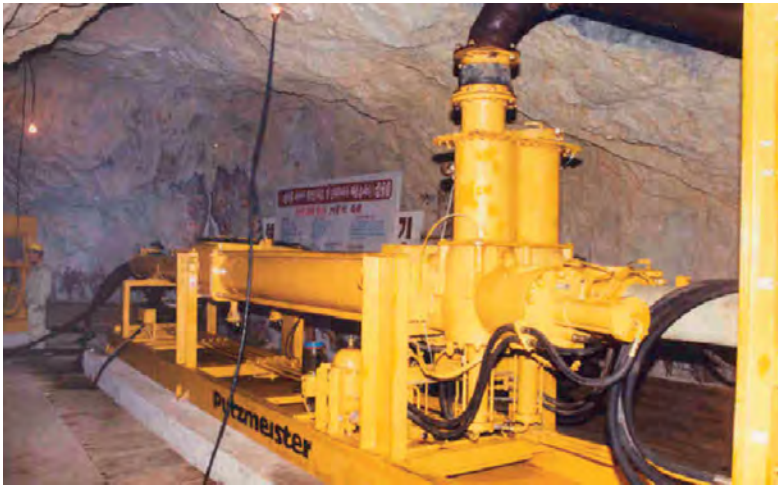
Fig. 60: Seat valve pump with mounted damping vessel
