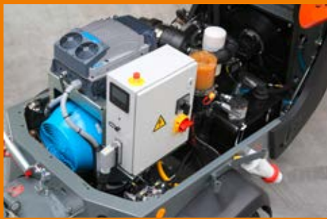
Powerful compressor unit with frequency-controlled electric motor
