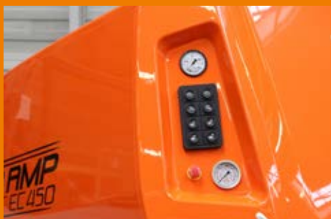
Straightforward operating panel with simple, robust keypad and two pressure gauges
