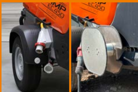
Simple connection with 63 A CEE outlet via provided 63 A cable
