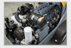
Oil-cooled 4-cylinder Deutz diesel engine with an efficient compressor for maximum pump output, and enough reserve power for more challenging jobs
