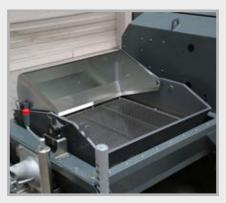
Conveyor with a volume of 250 I, a larger filling area and a swinging spray guard — with a powerful vibrator as standard. Lower filling height facilitates final cleaning and loading by truck mixer.
