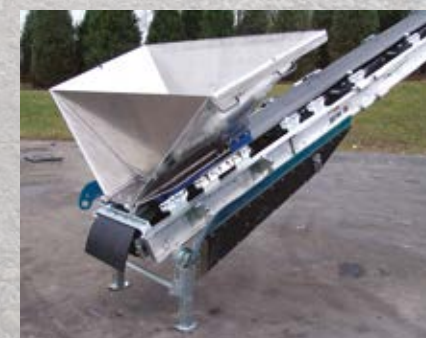
Front end loader hopper 2,00 m x 1,00 m (Optional)
