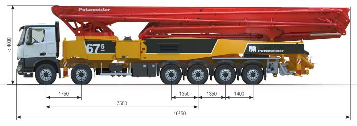
Note: Standard version. Dimensions and weights depend on truck, pump model and equipment. Dimensions in mm. For illustration only.
