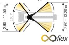
Dimensions can differ depending on configuration. Support width based on center of support leg. The specified values are reference forces.
