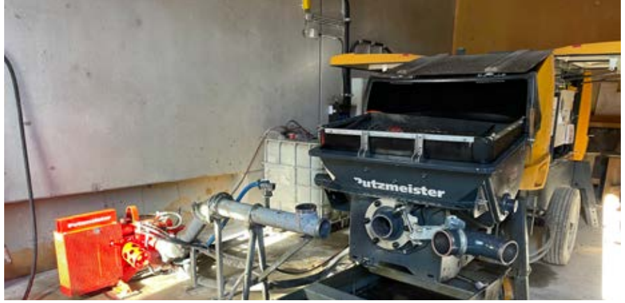
Stationary concrete pump BSA 1408 E with gate valve, hinged elbow and T-piece for simpler cleaning, cleaning tank for cleaning the hopper
