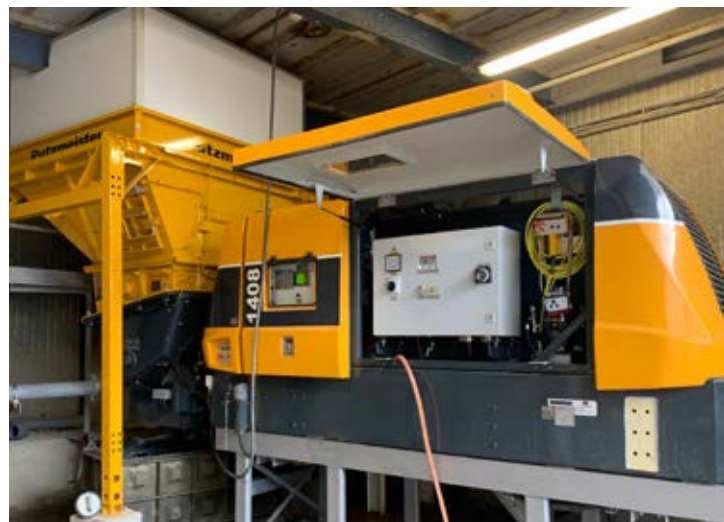
▼ Stationary concrete pump with extension hopper under mixing plant
