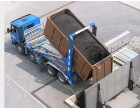
LKW receiving silo
