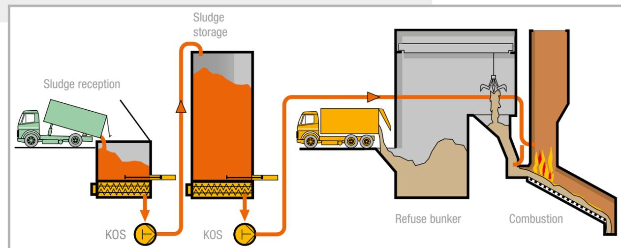
As only approximately 10 – 15 % of the total material incinerated is sewage sludge, the fluctuating consistency of the sludges (they generally derive from different sewage plants) has no important influence on the process of incineration.
