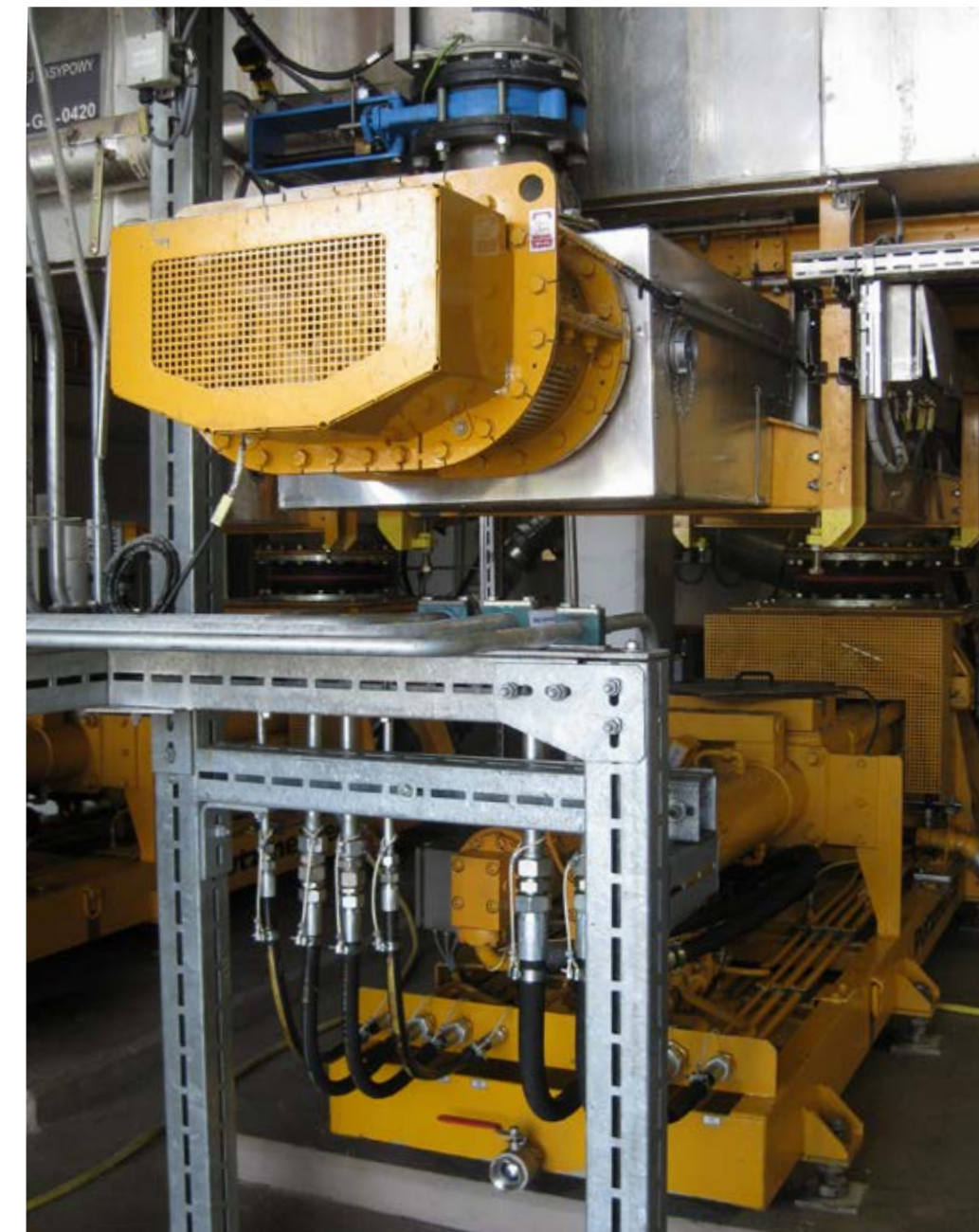
Twin feeding screw SHS 1732 SH to feed hot sludge into the KOS piston pump. Full dried sludge dosing at the rear end of the twin feeding screw.
