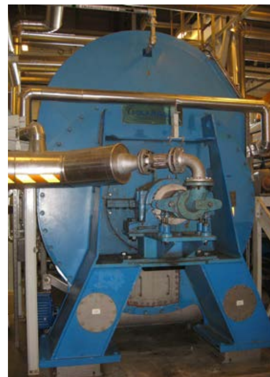
Twin feeding screw SHS 1732 SH to feed hot sludge into the KOS piston pump. Full dried sludge dosing at the rear end of the twin feeding screw.
