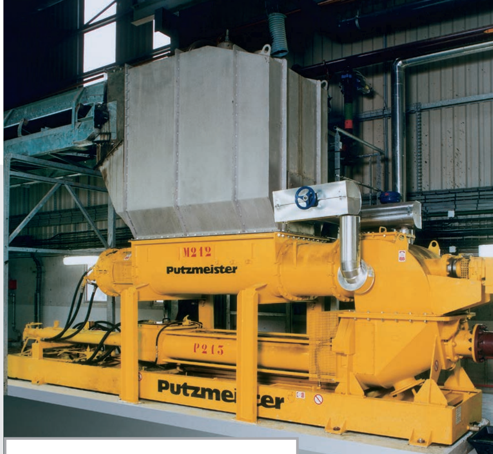
Biowaste recycling plant in Varenne-Jarcy, France: KOS 2180 pumping biomass material into a fermentation plant
