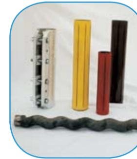
2. Unlike most "threaded" tubes, the S5 uses a spacer plate and tie rod system for quick and easy removal. This allows different size stator tubes to be used on the same machine.
