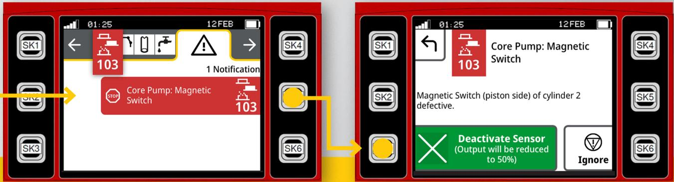
Clearly guided fault management on the radio remote control and the graphic display
