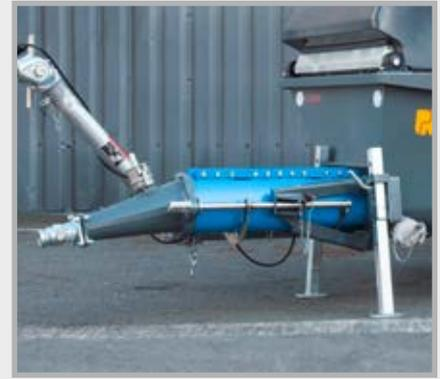
The patented quick-change system for the worm pump saves time and facilitates the handling. Without additional tools only one person is needed to change even the the heaviest 2L8 rotor/stator combination.
