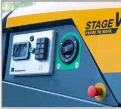
The control panel with an intuitive keypad increases operational safety. A simple to understand display behind scratch-resistant glass provides the user all relevant information.
