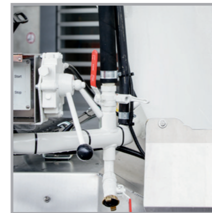
Easier accessibility and greater clearance, even with short wheelbases, are provided thanks to the water line integrated in the ladder hook.
