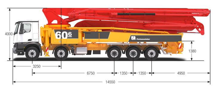
Note: Standard version. Dimensions and weights depend on truck, pump model and equipment. Dimensions in mm, MB-Arocs 4545K, Euro 3. For illustration only.
