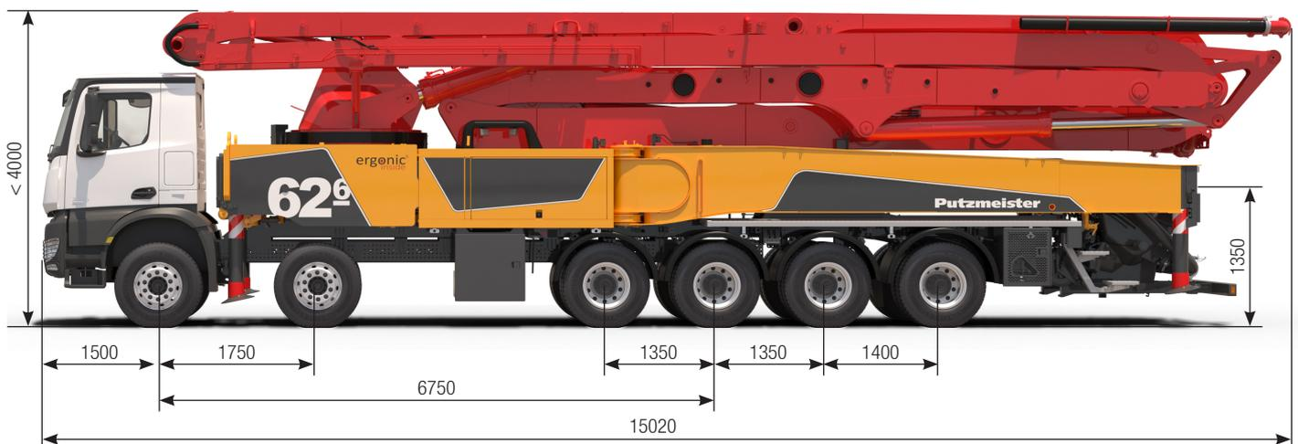
Note: Standard version. Dimensions and weights depend on truck, pump model and equipment.
