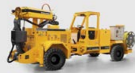
SHOTCRETE EQUIPMENT 4 – 30 m³/hr Horizontal Reach: 7 - 15 m Vertical Reach: 7.5 - 17 m
