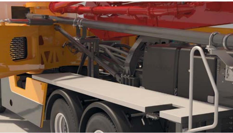
The new I frame concept offers improved torsional properties in comparison to the fixed frames. It has the same elasticity as the chassis. Driving thus becomes a pleasure and service life of the vehicle is extended.
