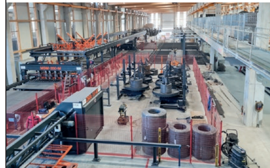
Mesh welding machines for box culverts, precast concrete elements and customer-specific meshes
