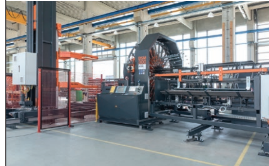
Cage welding machines for manhole and concrete pipe reinforcements
