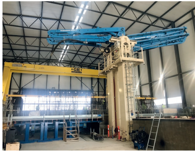
Fig. 5 and 6: Reinforcement cage of the first foundation element (left) and the two MX24 distribution masts on the tubular column system (right).
