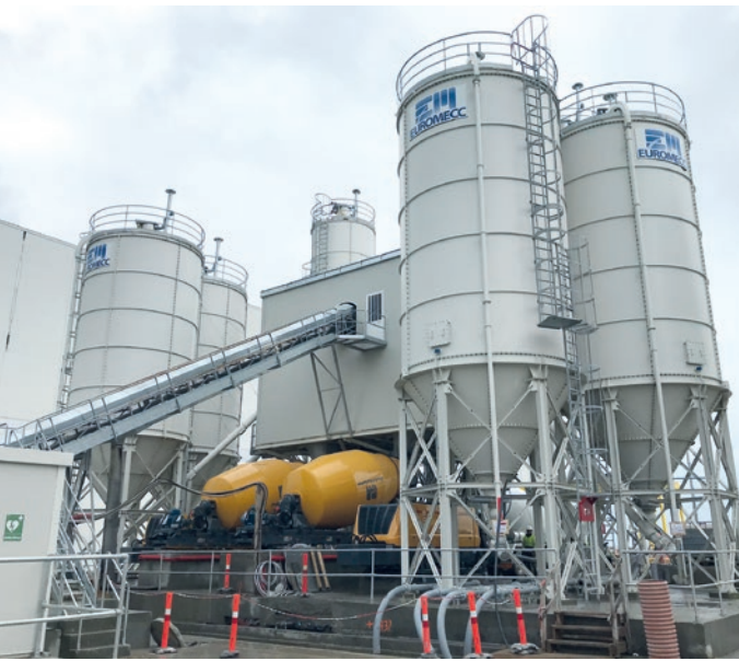
Fig. 3: Two mixing plants with the 8 m 3 buffer tanks and stationary concrete pumps BSA2109 H E.
