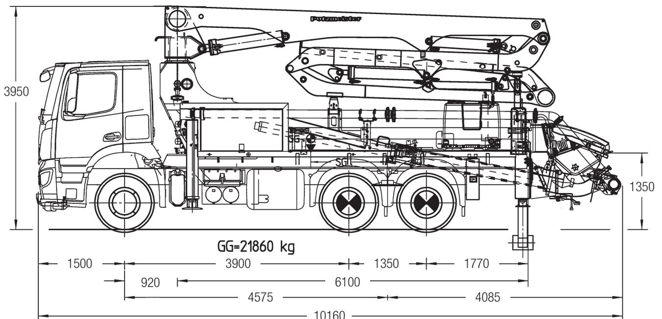
Note: Standard version on 3 axles. Dimensions and weights depend on truck, pump model and equipment.
