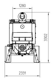
Note: Standard version BSA 14000 HP D. Dimensions and weights depend on equipment. Subject to technical modifications and errors.
