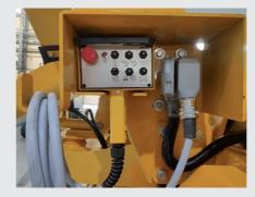
The equipment's rear functions can be controlled remotely through the **cable**
