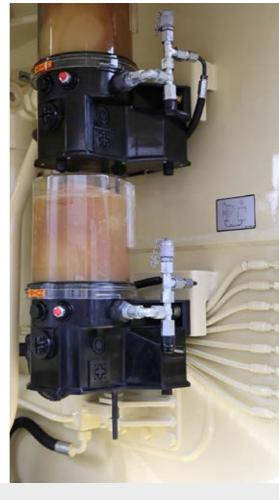
Combined centralized lubrication system:
