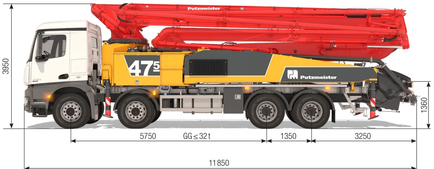
Note: Standard version. Dimensions and weights depend on truck, pump model and equipment.
