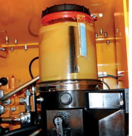
Automatic lubrication system of the concrete pump for proper machine maintenance
