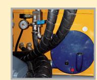
Liquid additive pump, synchronized with the concrete flow.
