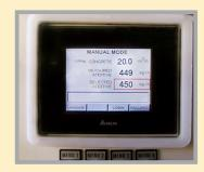
Control system with multilingual colour display, indicating concrete flow, additive dosage, faults, diagnoses and alarms.
