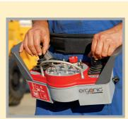
Proportional remote control for easy handling of arm movements, dual use (radio/cable).
