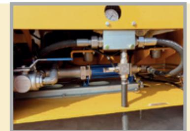
Screw additive pump with flowmeter
