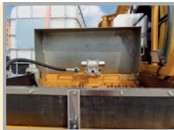
Hopper with agitator, electric vibrator
