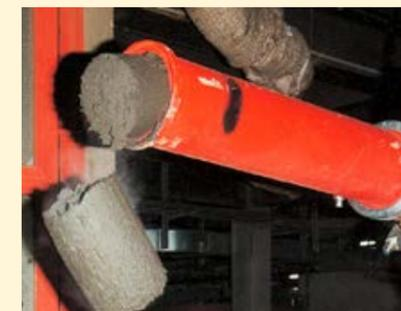
Sewage sludge from filter press and centrifuges
