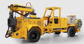
SHOTCRETE EQUIPMENT 4 – 30 m³/hr Horizontal Reach: 7 - 15 m Vertical Reach: 7.5 - 17 m
