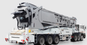
TELEBELT Horizontal Reach: 31.8 – 61 m Vertical Reach: 16.78 – 34.70 m
