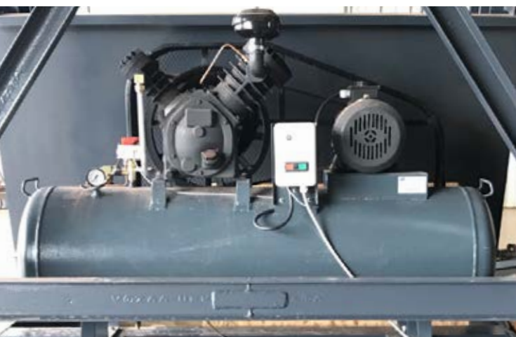
#8 Working pressure of up to 9 bar thanks to Double Stage Air Compressor
