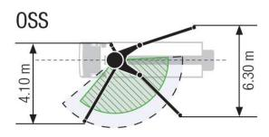
Support width based on center of support leg
