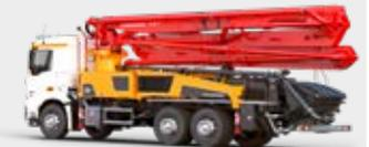
TRUCK-MOUNTED CONCRETE PUMP
