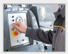
The easy to read, analog instruments and robust switches are protected by a sturdy flap against dirt and the risk of being damaged.
