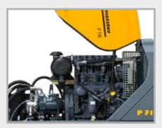
Reliable oil-cooled 3-cylinder Deutz diesel engine complies with exhaust emission regulation (Stage 3A).
