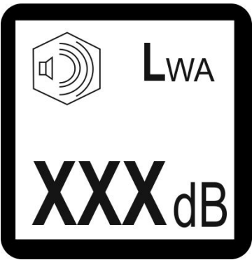
Figure 7: Plate – sound power level
