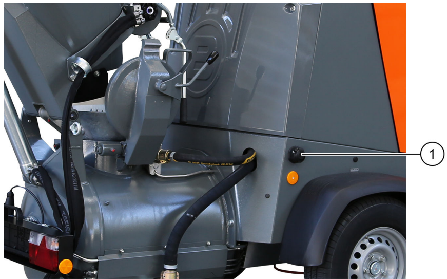
Figure 41: Lighting equipment socket
