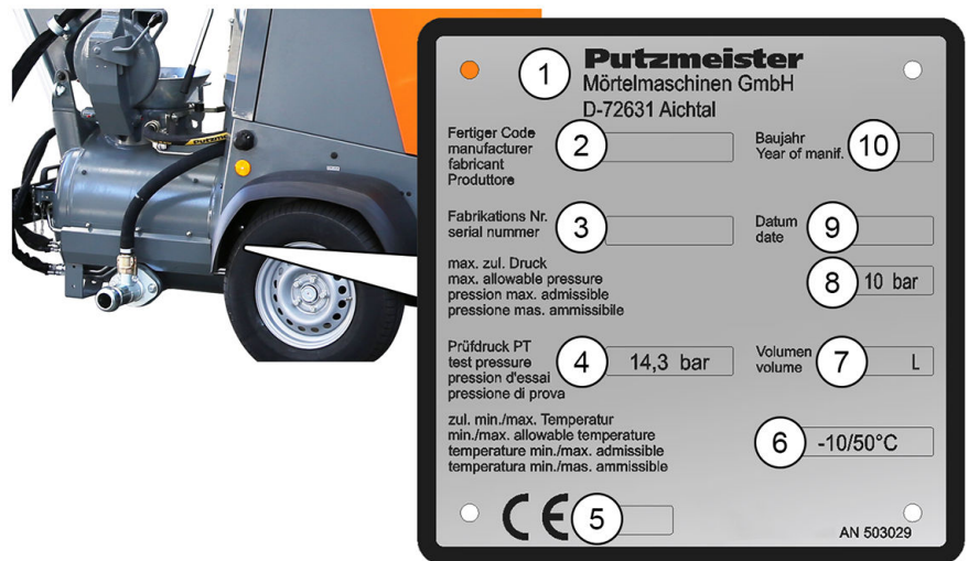
Figure 6: Mixing vessel rating plate
