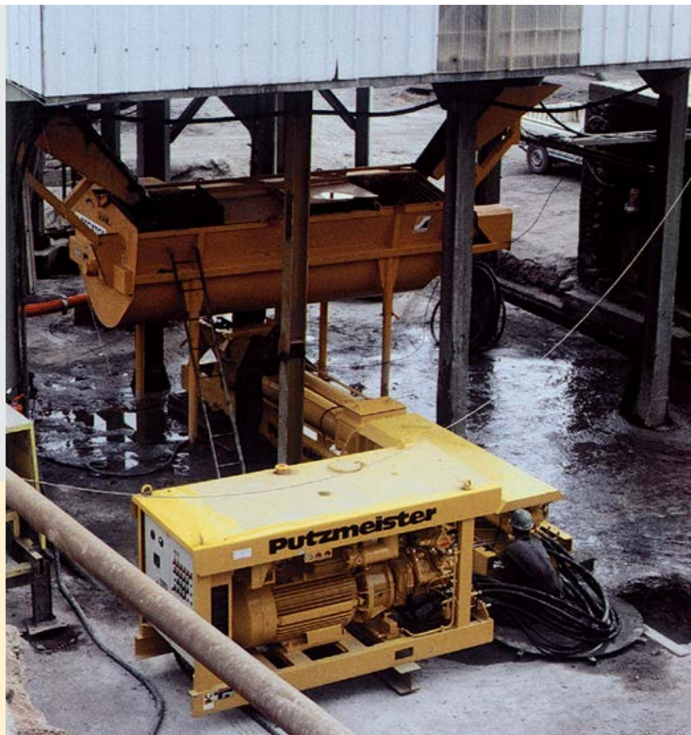
Directly above the solids handling pump KOS 2180 is the 12 m 3 capacity supply container. The hydraulic unit of the solids handling pump is in the foreground.
