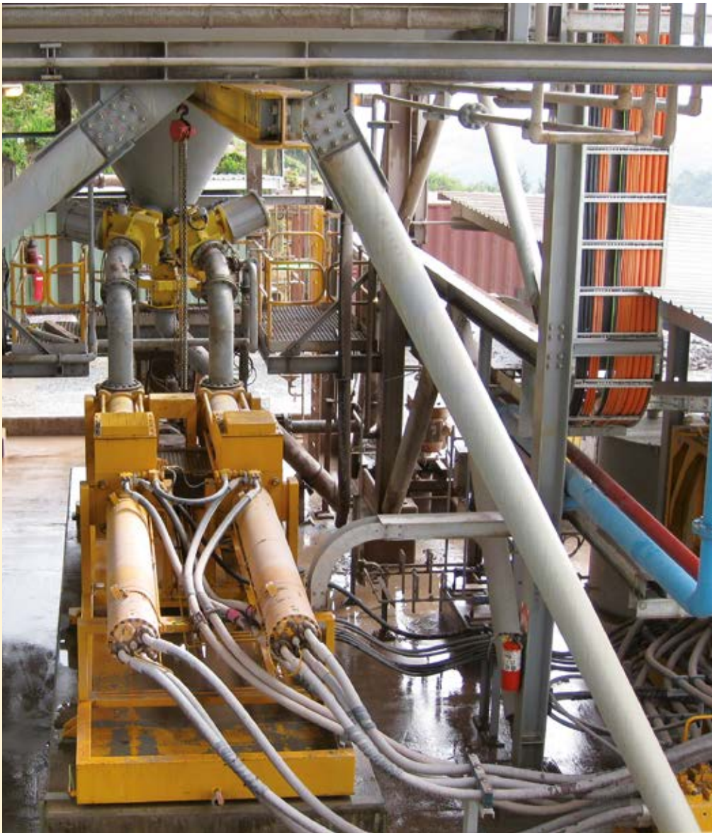
HSP 25100 HPS double piston pump with PCF Control
