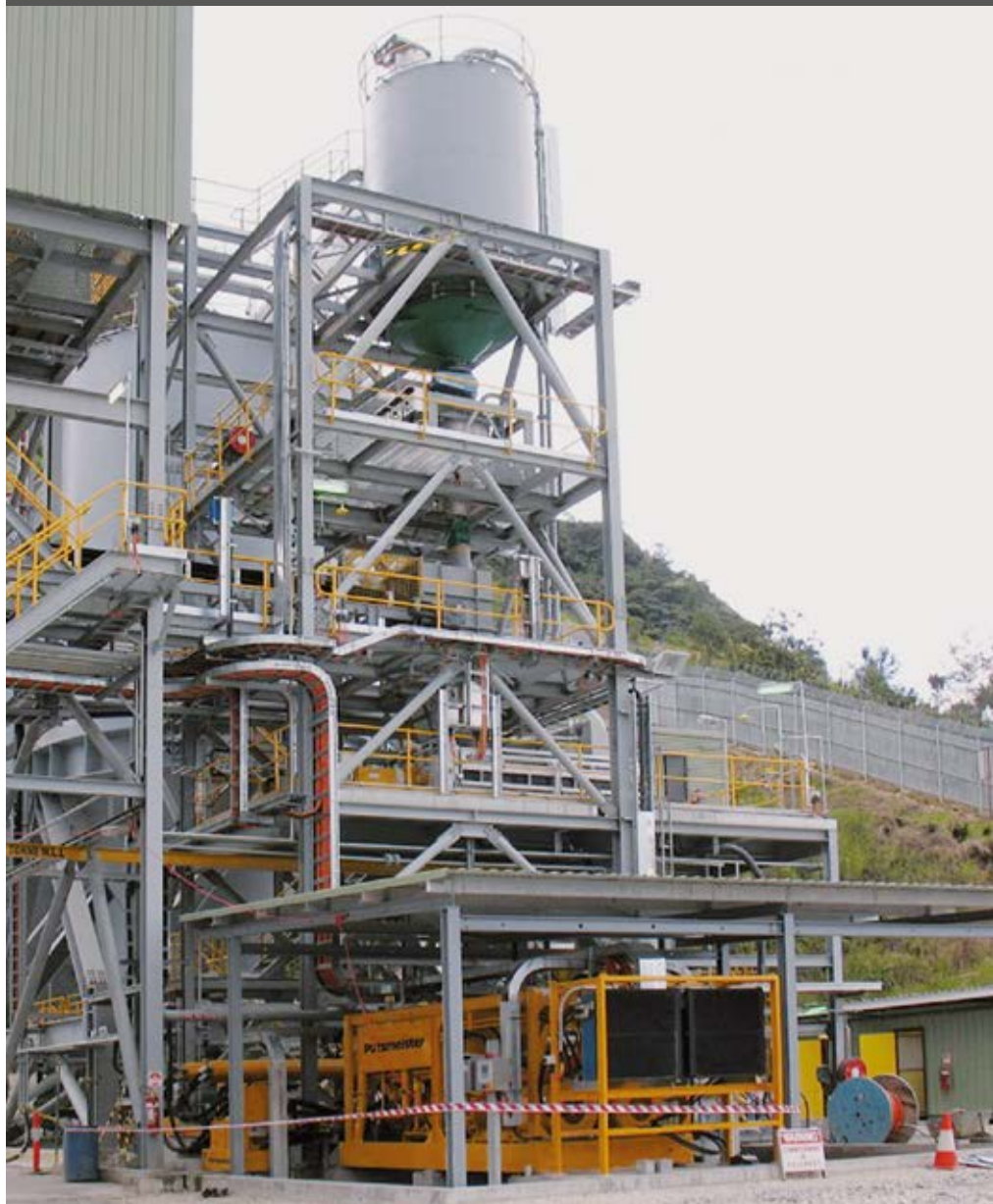
Preparation and pumping plant for the backfill material. Power pack HA 800 E (2 x 400 KW) to drive the HSP 25100 HPS.
