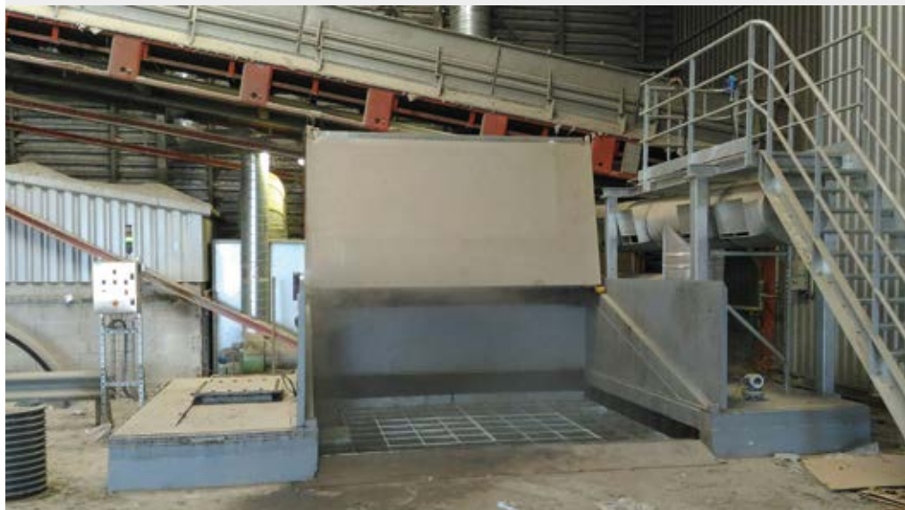
Sludge receiving bunker with typical Putzmeister A-fold lid
