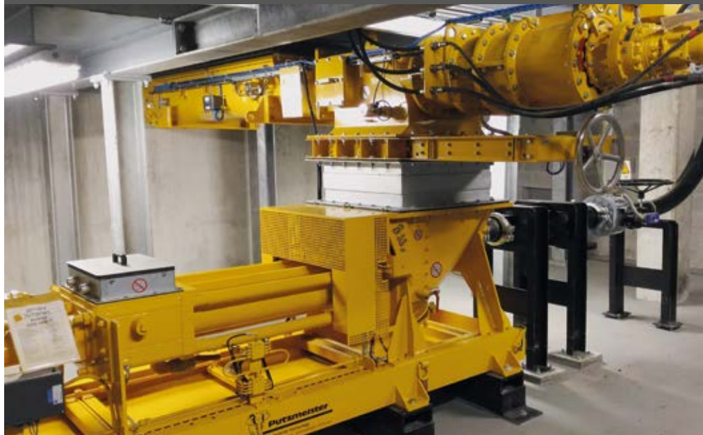
Silo discharge screw SHS 3132 SH feeding the KOS 1040 double-piston pump with S-transfer tube
