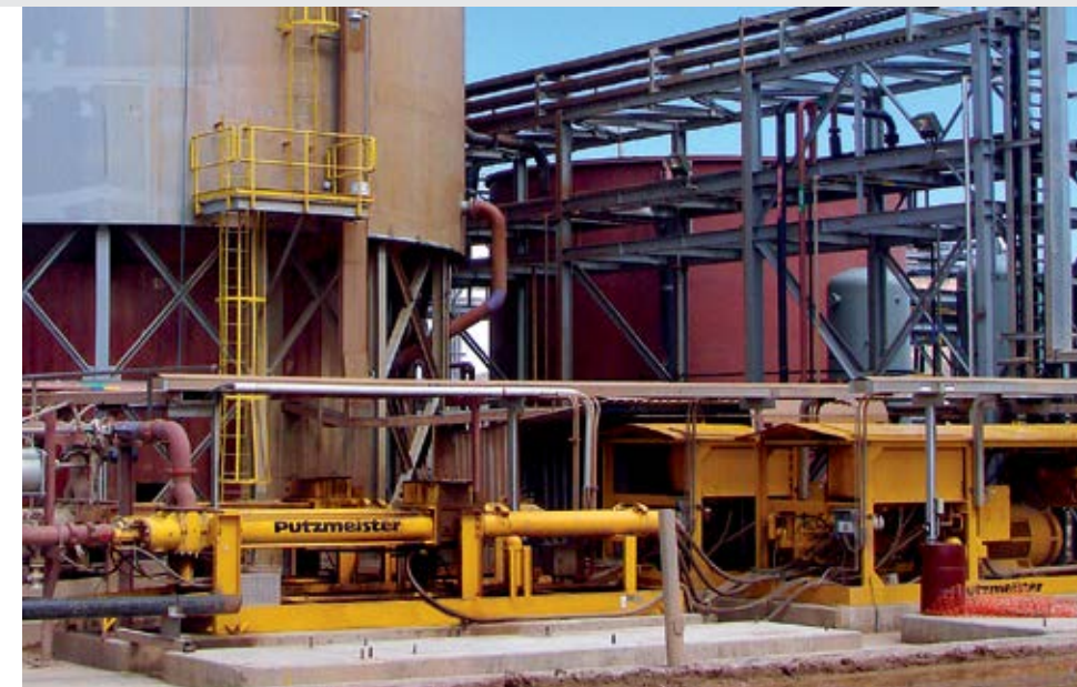
HSP 25100 HP - High performance pump for mining tailings and fly ash
