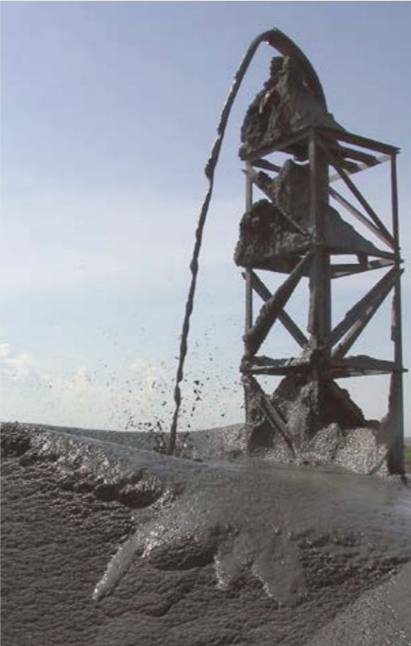
Tailings pond with discharge pipe and tower
