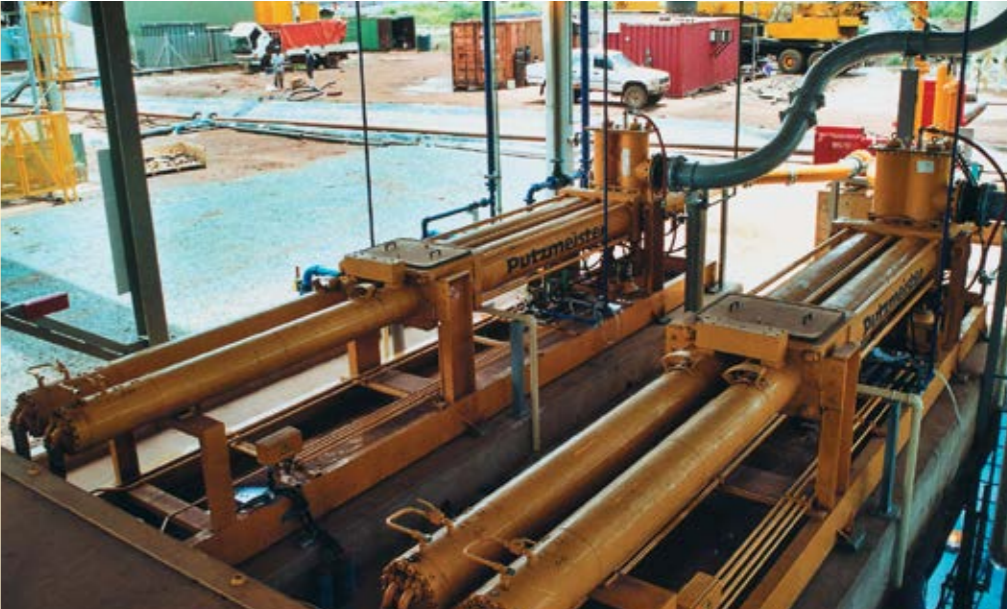
Two HSP 25100 with suction connection and low pressure damper
