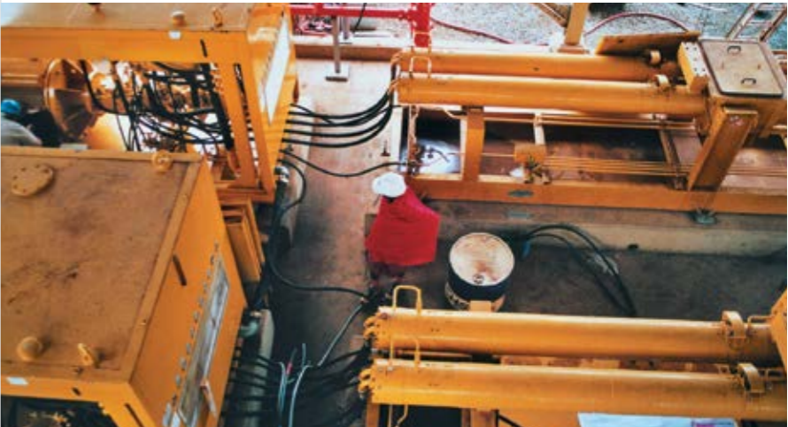
The two HSP 25100 pumps are each driven by a HA 315 E
